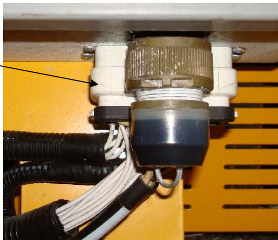
Figure 7-3. Ground Control Panel Receptacle
